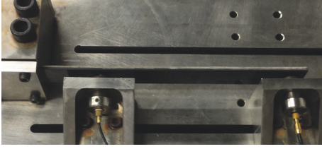
FIGURE 1: The Oberst beam test bench.
